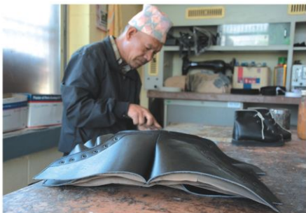
Individualised clubfoot shoe is being manufactured at HRDC
