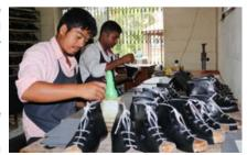
Fabrication of ortho shoes at HRDC
